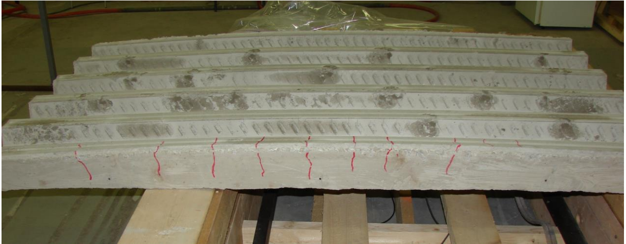
Figure 8: Uniformly distributed cracks in concrete after finishing the test and removing of steel sheeting.
