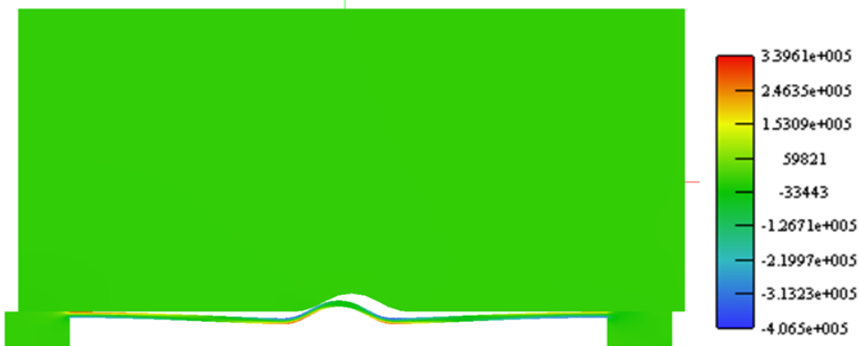
Figure 2: 2D model: deformed sheeting corresponding to slip 2 mm; displayed stress in longitudinal axes [kPa].
