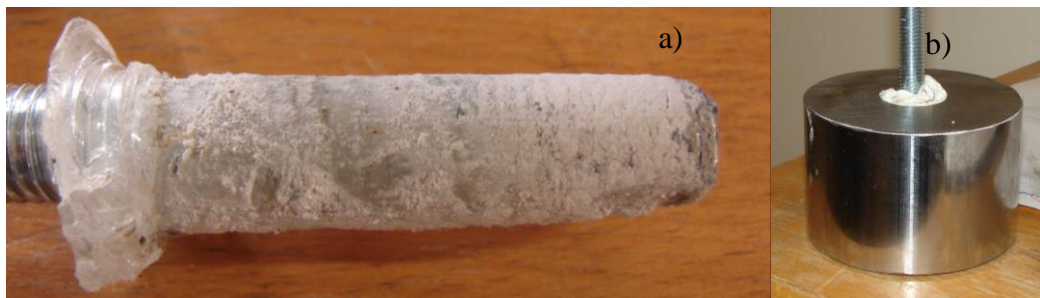
Figure 2: a) M12 specimen after failure (epoxy resin). b) steel specimen
